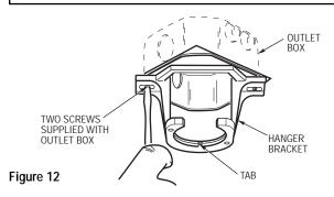
2. Carefully lift the fan and seat the hanger ball/downrod assembly on the hanger bracket that was just attached to the outlet box (Figure 13). Be sure the groove in the ball is lined up with tab on the hanger bracket (Figure 12).
